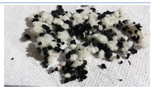
The OWB Cement Control Additive creates an impermeable seal to stop losses.
